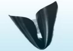
BR 287 Flexible Borated shielding material can easily be handled and installed by nonspecialized personnel. It is readily applied to concrete & metal surface or other wall materials using standard mounting technique. This flexible material can be cut and shaped using an ordinary knife and scissors. This material can be molded or extruded like Tubing, bushing, gasket, any cross section profiles and parts as per your Drawing and requirements
